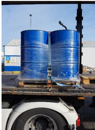
Variante 1 mit Drumclip, handgewickelt / Variant 1 with drumclip, manually wrapped
