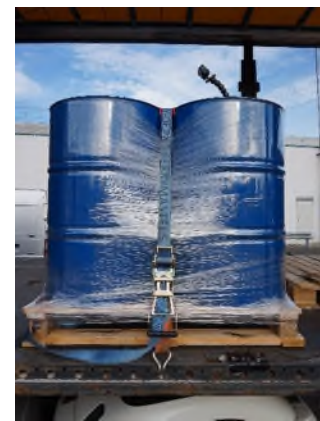
Variante 3 mit Drumclip, maschinell gewickelt / Variant 3 with drumclip, mechanically wrapped
