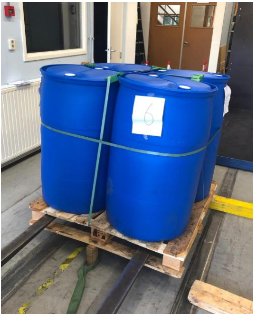
Figure 7. Set-up Rotational Edge Drop Test
