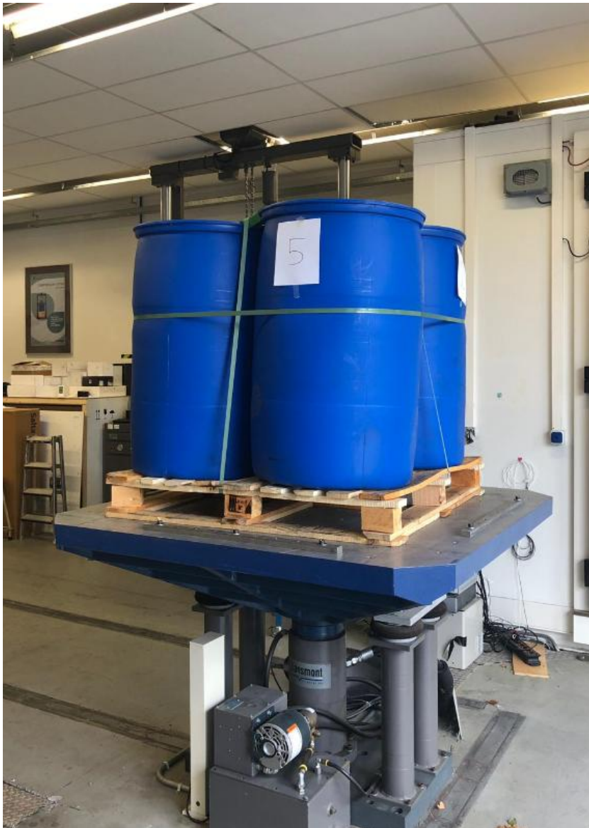
Figure 6. Test setup for vibration test
