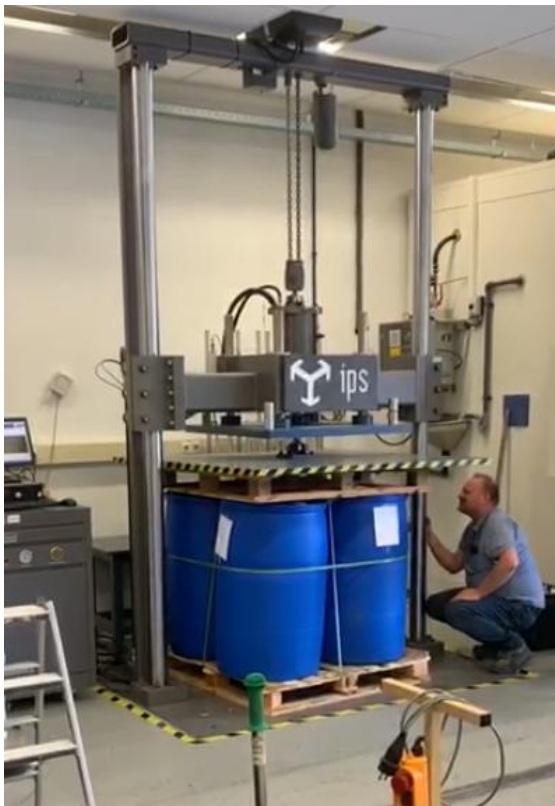
Figure 5. Set-up compression test
