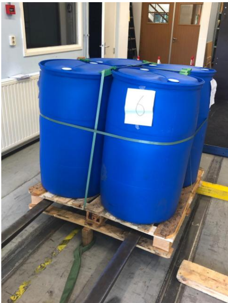
Figure 4. Set-up Rotational Edge Drop Test
