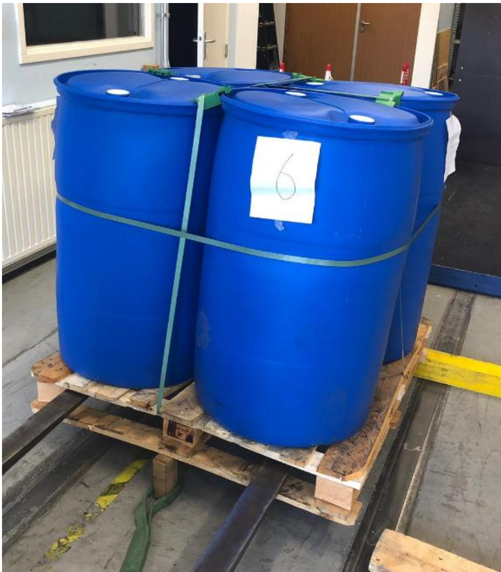
Figure 8. Position of drum clips during drop testing.
