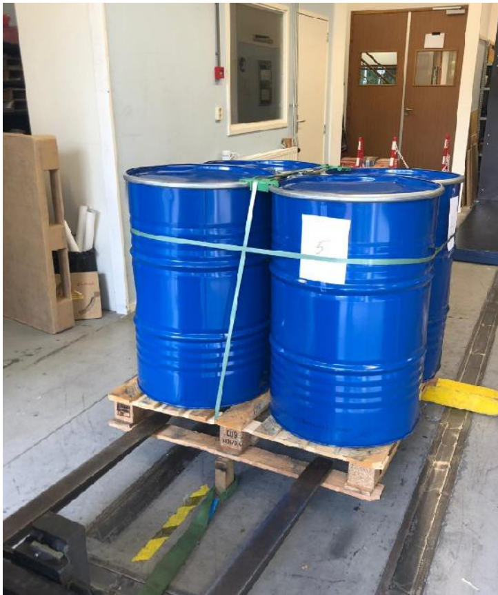
Figure 7. Set-up Rotational Edge Drop Test
