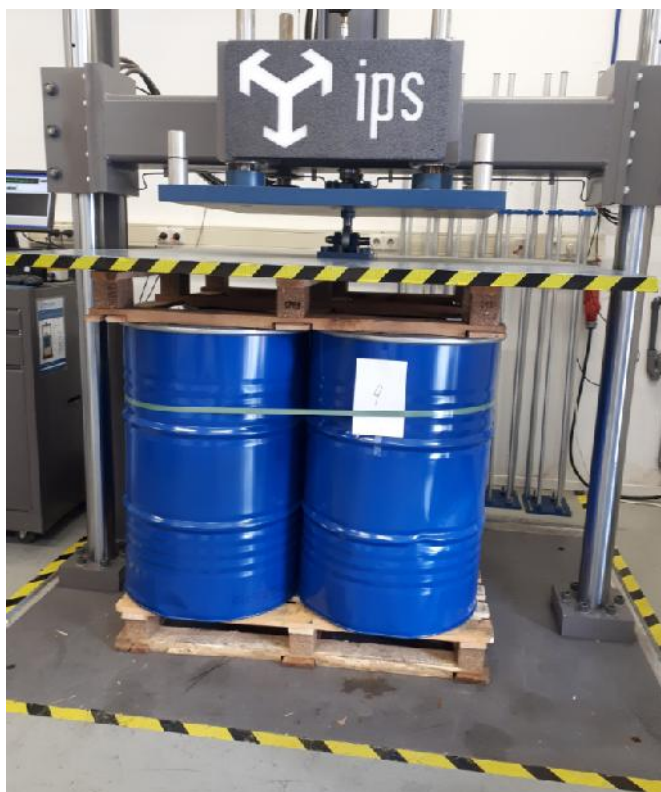
Figure 5. Test set-up Compression Test
