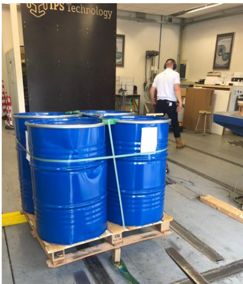
Figure 4. Set-up Rotational Edge Drop Test
