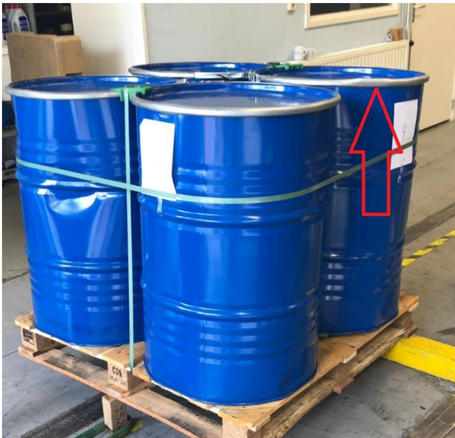
Figure 8. Damage to drum ring; only face 4.
