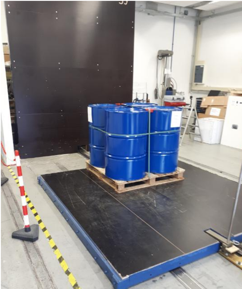
Figure 3.DUT on horizontal impact tester.
