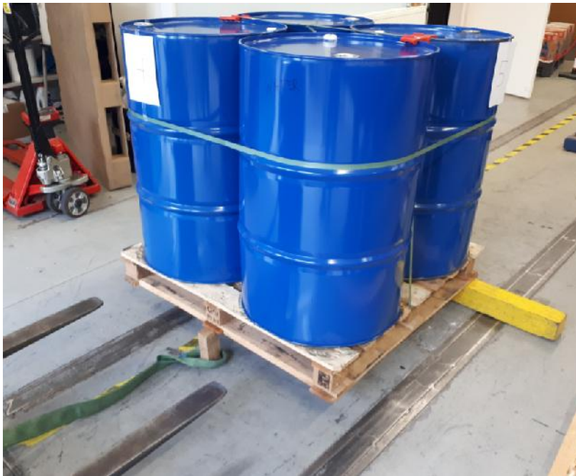
Figure 7. Set-up Rotational Edge Drop Test
