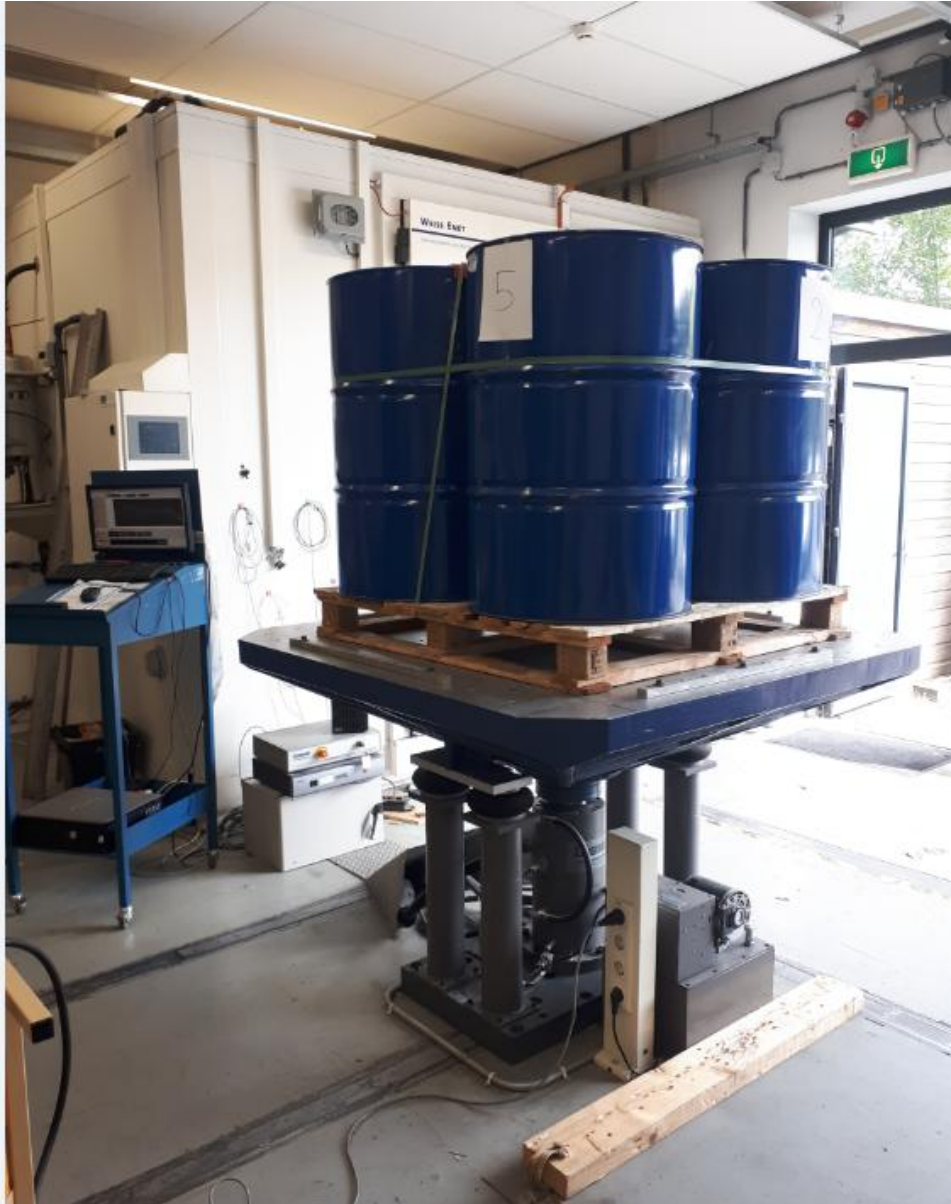
Figure 6. Test setup for vibration test
