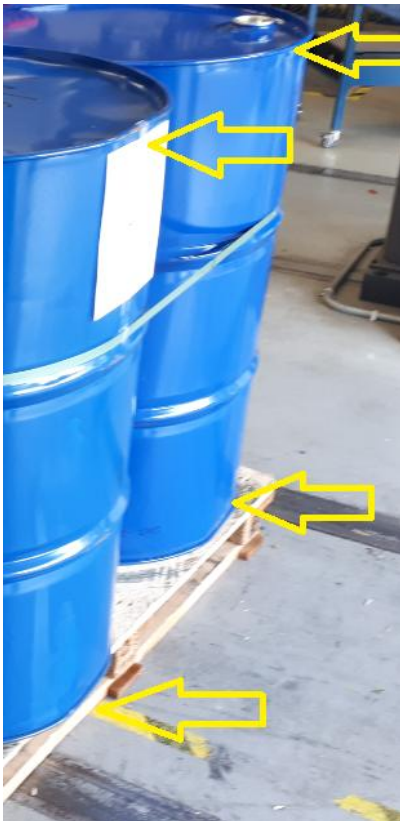
Figure 8. Damage to drums; only face 4.
