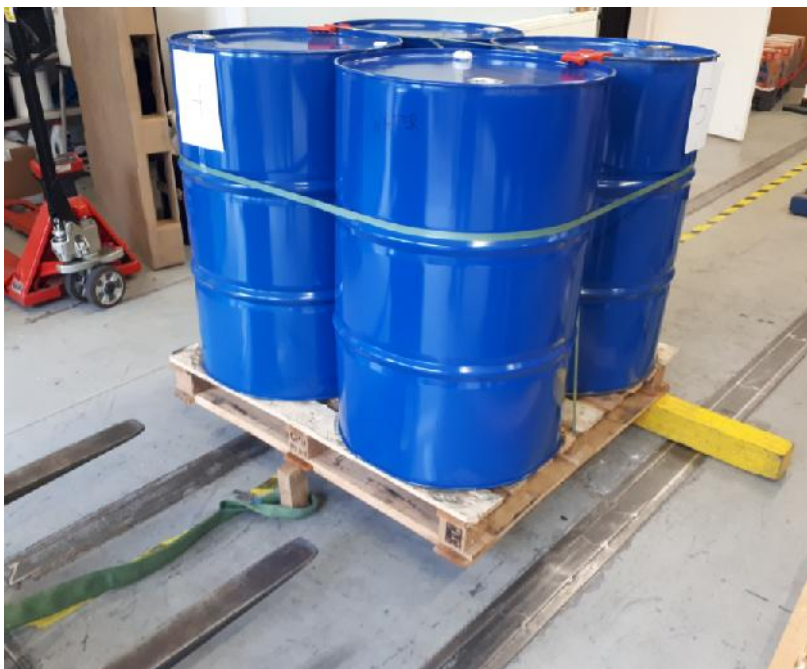
Figure 4. Set-up Rotational Edge Drop Test
