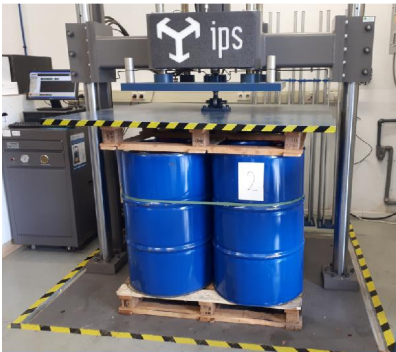
Figure 5. Test set-up Compression Test
